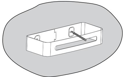
Using the basket as a template, mark the positions of the screw holes.
