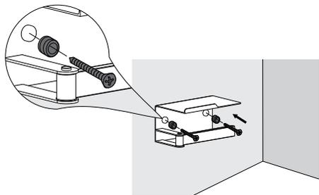
Screws go through the nuts and screw the product onto the wall.
