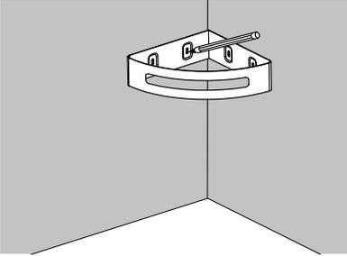
Using the basket as a template, mark the positions of the screw holes.
