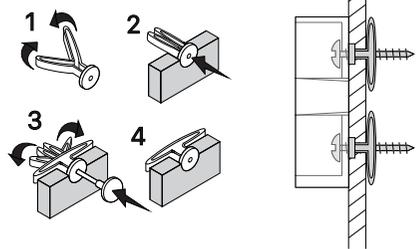
Drill 5/16" holes, Use the anchors to secure the basket.
