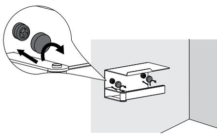
Tighten the decoration cap onto the nuts after fix the products.
