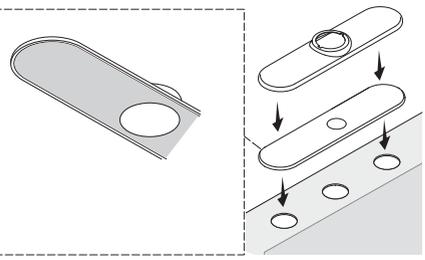
Place stainless (non-staining) deck plate and deck plate gasket onto sink, secure it with silicone. **Note: the deck plate need purchase seprately.**
