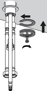
From underneath the countertop, Slide rubber washer, metal washer and mounting bracket onto the thread shank.
