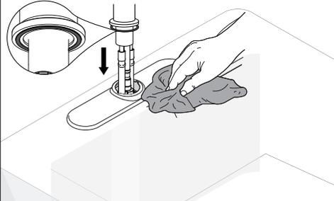
Put the rubber O-ring into the bottom gap of faucets then Insert faucet into faucet hole.
