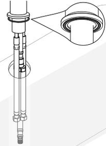
Put the rubber O-ring into the bottom gap of faucets then Insert faucet into faucet hole.
