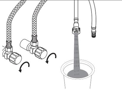
Turn on water suppliers. Place a bucket below outlet tube, slowly open and close the supply angle valves, **This will prevent debris from being lodged in the hose and sprayer.**
