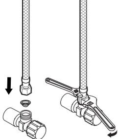
Connect and tighten the supply hoses by using two adjustable wrenches (avoid twisting or kinking).
