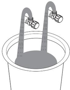
Shut off water suppliers. Remove the old faucet, clean the mounting surface.
