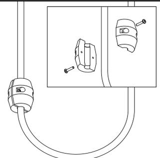
Install the hose weight on the outlet side of the hose, near the loop.
