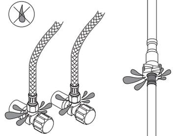
Turn on the water suppliers, Shut off the faucet and check for leaks.
